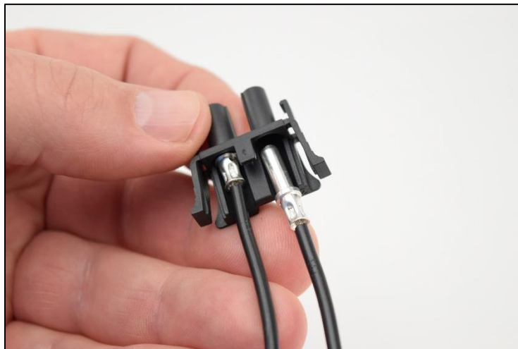
Step 3: Insert crimped contacts into body
