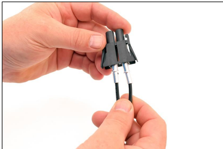
Step 3A: Insert contacts into body
