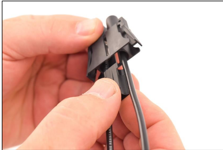
Step 4B: Fit between wires
