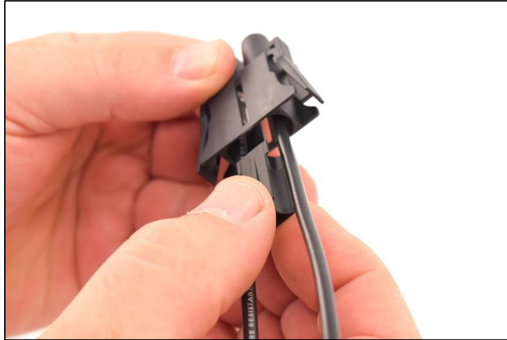
Step 4B: Fit between wires
