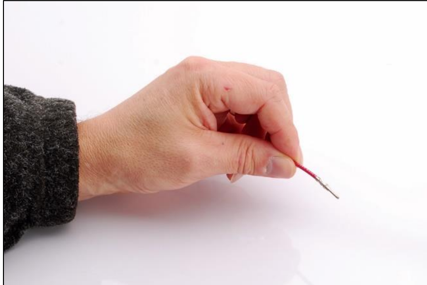
Step 1: Grasp crimped contact approx. one inch behind the contact barrel.
