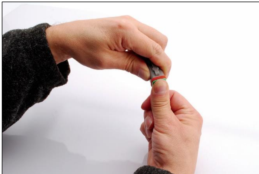
Step 5: A 'click' will be felt when the wedge is fully installed.
