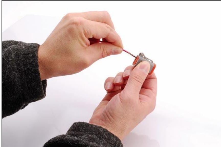
Step 2: Hold connector with rear grommet facing you.
