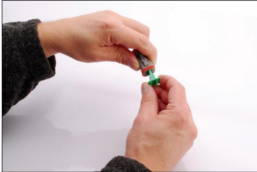
Step 4: Insert wedge into connector.
