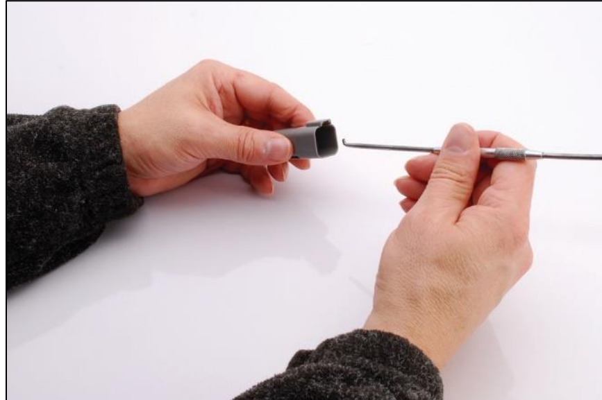
Step 1: Remove wedge by inserting a hook into an opening of the wedge.
